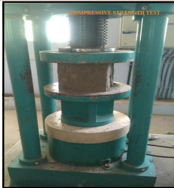
FIGURE 5: EXPERIMENTAL SETUP FOR CS TEST
